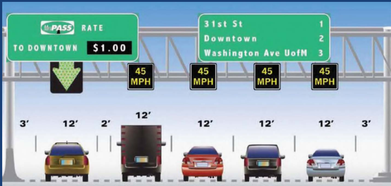
Minnesota I-35W Planned Overhead Signage Showing Priced Dynamic Shoulder Lane and Variable Speed Limits
