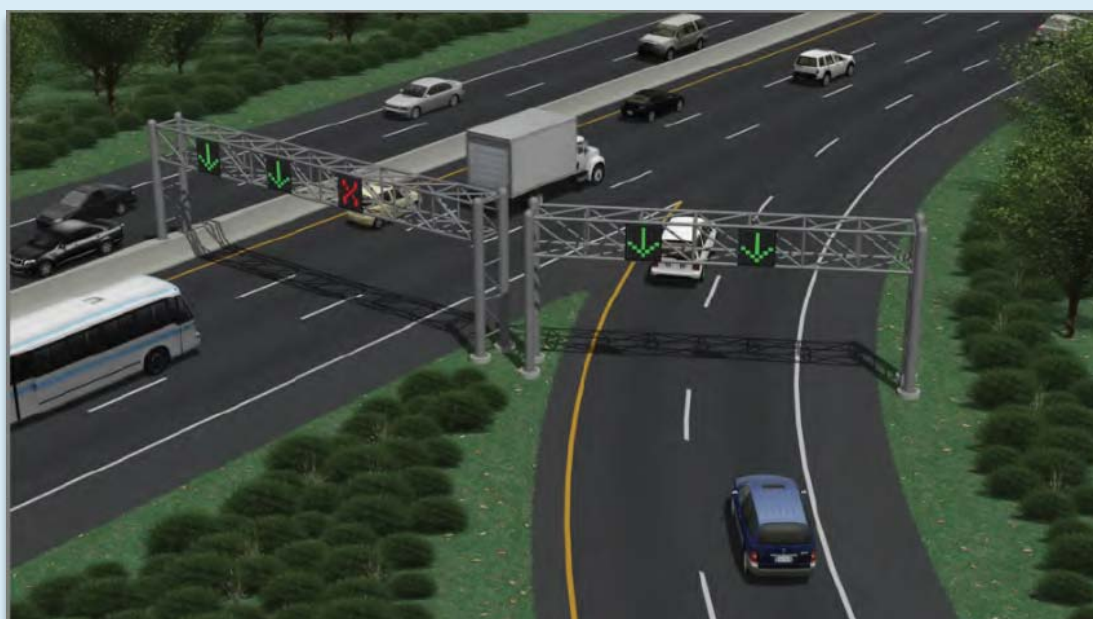
Figure 12. Simulation graphic. Dynamic junction control implementation.
