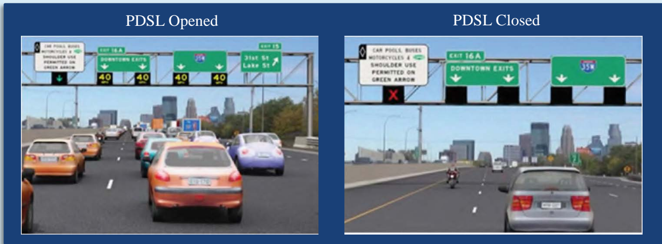
Figure 4. Simulation graphics. Typical Section of MN I-35W Northbound Priced Dynamic Shoulder Lane (PDSL).
